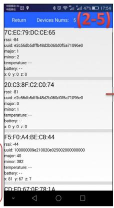
Click the Searching on the up left corner will enter into this page, then can check the numbers of the online devices, MAC address ,RSSI, UUID, M AJOR, MINOR, battery level, temperature, 3 axis sensor value3 (Temperature and 3 axis sensor are only for the customized
